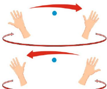
To turn on the fan or increase fan speed, move your hand from left to right several times. With each hand gesture, the colour of speed indicator will change.
